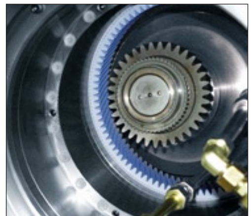
Vitrified bonded ring for Prävema High Performance Gear Honing
